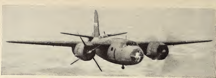
A B-26 flies safely with one motor stalled and the blades feathered.
